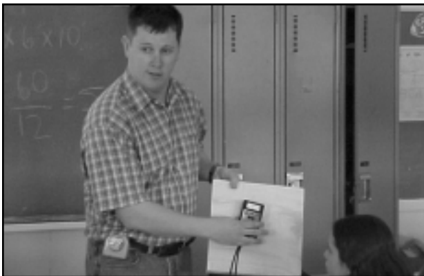
Brad Dillon using a device to measure the percentage water content of a board.
